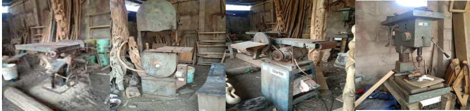
Plate 1: Circular Saw Machine Plate 2: Band Saw Machine Plate 3: Sand Paper Machine Plate 4 Drilling Machine © Abiodun Idowu © Abiodun Idowu © Abiodun Idowu © Abiodun Idowu
